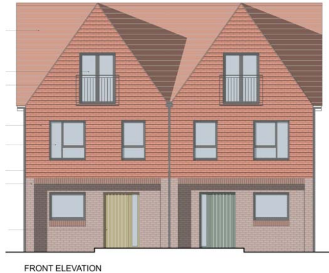
Figure 5-Front elevations of one pair of dwellings to the rear of the site
